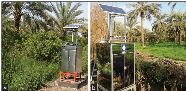
Fig 3. Light traps with solar energy (a- UK design, b- Iraqi design).
